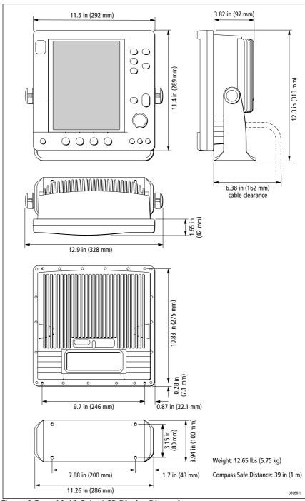
Figure 6-5: 10.4" Color LCD Display DImensions
